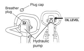
Figure 25. Removing Plug/Breather Cap
